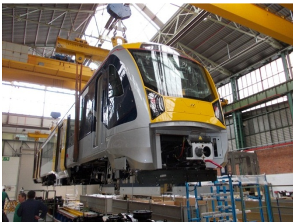
Fig 3: First vehicle being lowered onto bogie.
