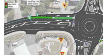
Capacity improvement and physical changes (Roundabout metering)
