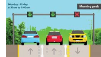
ITS intervention (Dynamic lane management)
