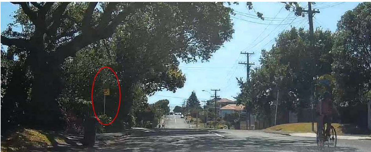
Figure 13: Speed table sign blocked by vegetation
