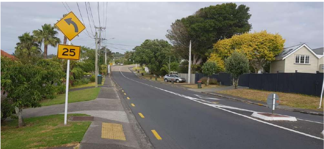
Figure 17: Incorrect advanced curve warning sign
