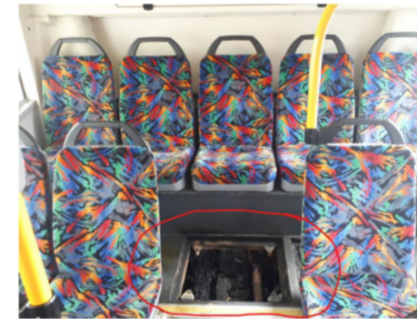
Interior of the vehicle unaffected. Access hatch opened by FENZ to extinguish the fire.
