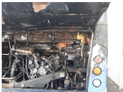
Extent of fire damage to the engine bay
