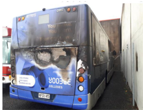
Extent of fire damage to the rear of vehicle
