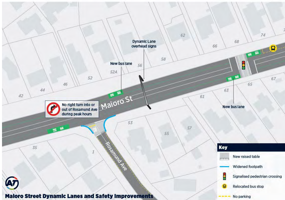
Diagram of proposed changes to Rosamund Avenue, includes the proposed signalised crossing
