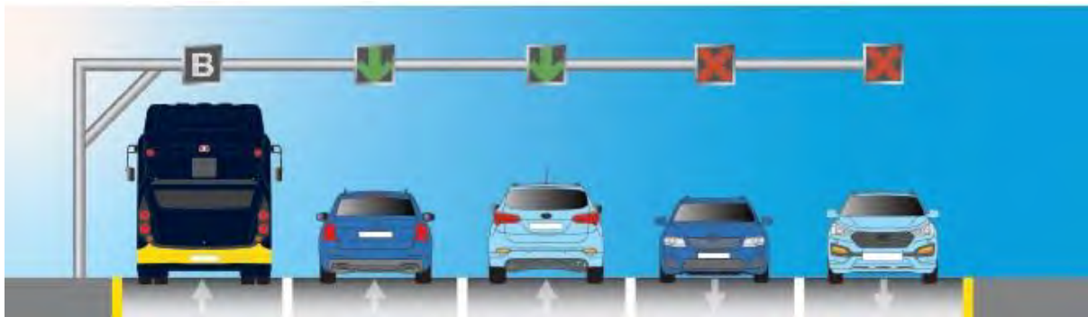
Diagram of the proposed dynamic lanes on Maioro Street in peak hours
